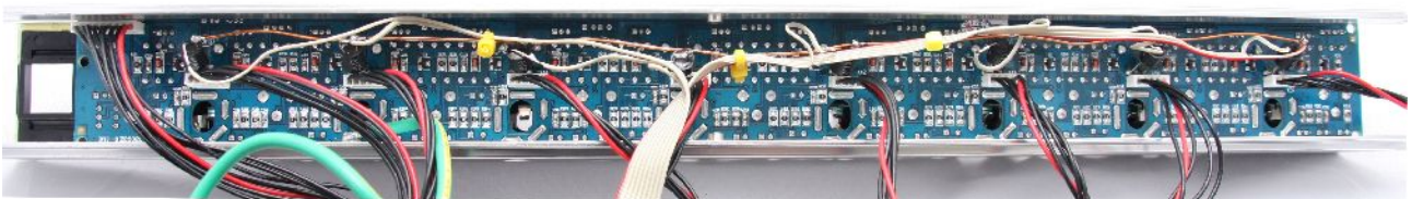
Picture 8: Finished front panel with couplers, anode wire and ribbon cable
