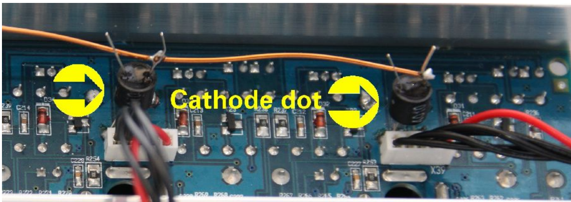
Picture 7: Couplers with common anode wire soldered
